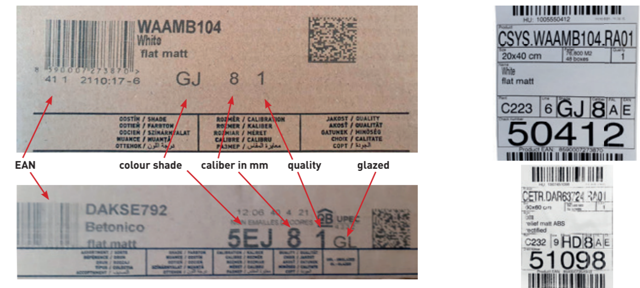
Fig. 1 Identification of the colour shade, size, quality, and typology (GL or UGL) is printed on a cardboard packaging and on a pallet.
